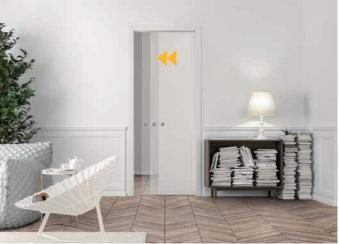
Thanks to the self-closing mechanism, once opened the door closes automatically. It is a mechanical system that can be installed also at a later time, on a pocket door system already mounted.
